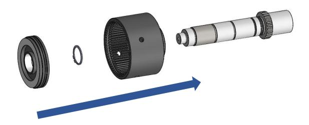
14. Spring, washer and segment should be assembled in a row.
