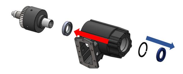
6. Segment and washer should be removed on the clutch shaft.
