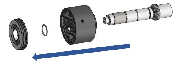
13. Piston and clutch shaft should be assembled in clutch case with segment after o-ring is changed and well greased.
